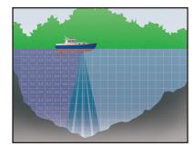
**Boat Mount:**Collect current profiles and discharge measurements from a moving boat or platform.
